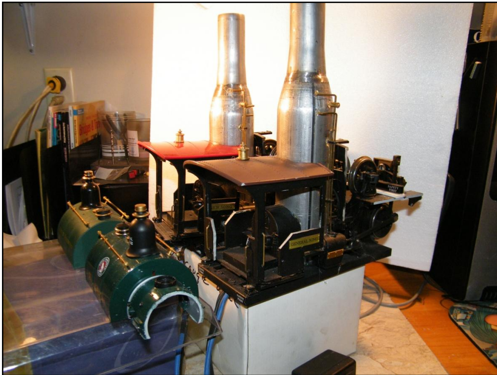
Two steam donkey units awaiting log skids & final detailing
